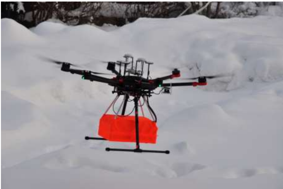
Zond-12e Drone 500A GPR system carried by the DJI M600 Pro drone in flight.
